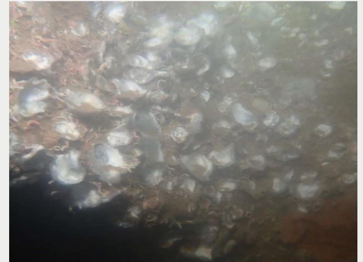
Unprotected Propeller (6 months after polishing)
