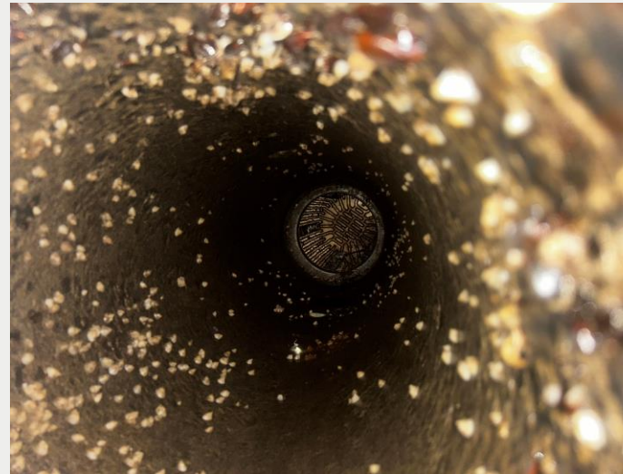
Picture A - With Sonihull (no visible organisms)
