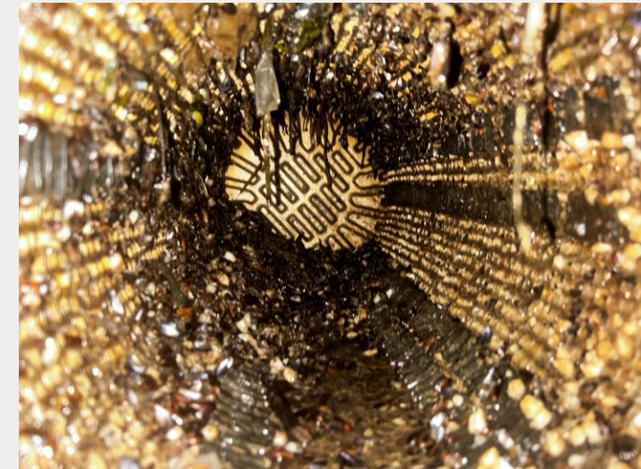
Picture B - Without Sonihull (clear organism buildup)
