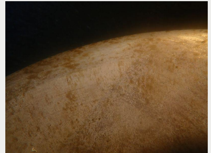
Sonihull protected Propeller (12 months after polishing)
